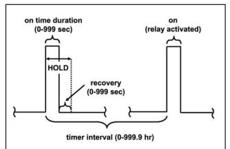
**FIGURE 5-3. Operation of the interval timer.** The numbers in parentheses are the allowed values for each timer parameter.
